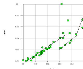
Figure 1: Data set of CR Compounds - Modulus 100 over Hardness
