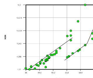
Figure 2: Data set of CR Compounds - Modulus 200 over Hardness
